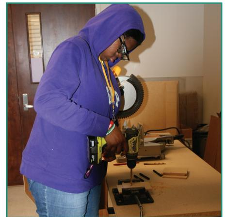
*WCHS student Kaliah O'Neal drilling pilot holes for the mechanical components of her box.*
