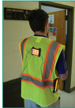
Gav is modeling the vest for a comfort test. (the exposed wires allow the unit to be removed when the vest needs to be laundered)
