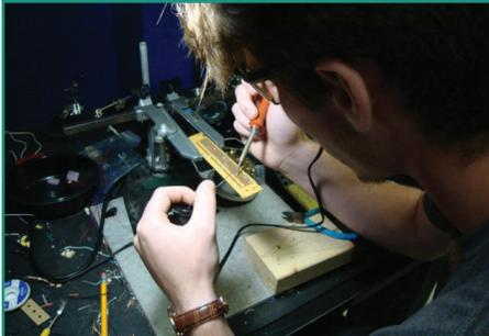
Gav Addison soldering one of the circuit boards that holds the LEDs.
